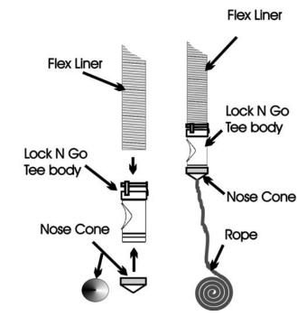
‡ NOTE: LOCK N GO TEE NOT REQUIRED WHEN INSTALLING WITH FIREPLACE INSERTS. USE THE "INSERT CONNECTOR". (See Fireplace Insert Installation below & Typical Installation # 3)
